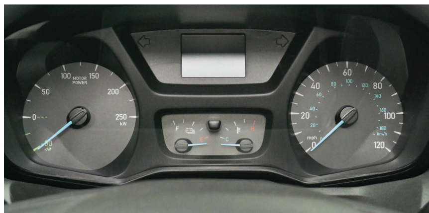
The dashboard of a Lightning Systems Ford Transit van, showing the power meter on the left, and the battery charge level indicator instead of the fuel gauge.
